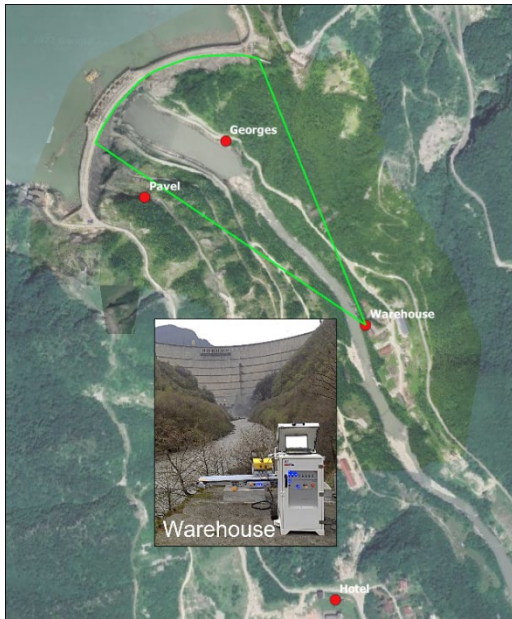
GBSAR installation concept at Enguri dam - Left: Longterm station – Right: Campaign stations
