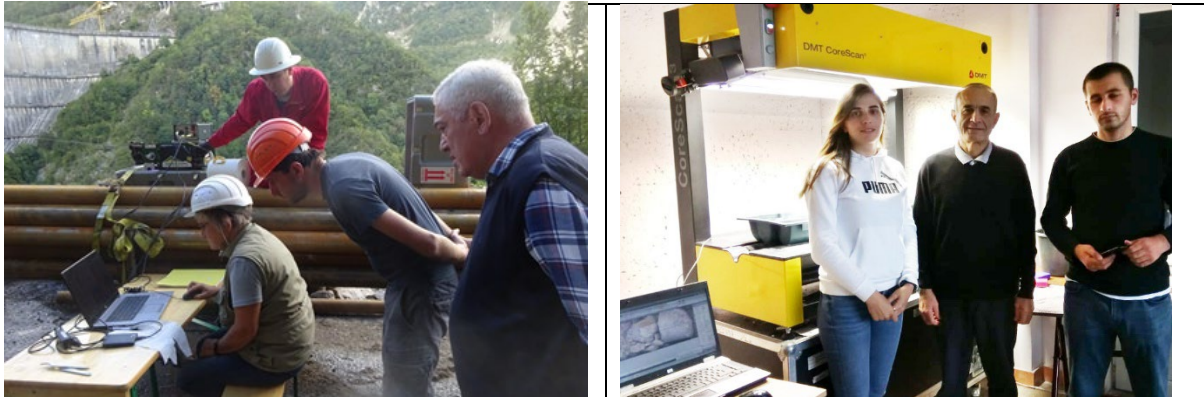
Left: Logging of Borehole KIT-1 with acoustic borehole televiewer (ABI). Right: Colleagues of GTU have been trained in scanning drillcores.
