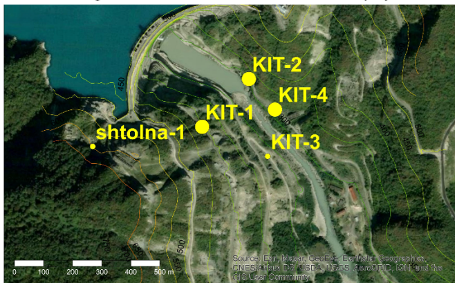
Fig. 1: Location of KIT-1, KIT-2, KIT-3, KIT-4 and Shtolna wells drilled as part of the project. The data of the two deep drill holes KIT-1 and KIT-2 were used for the evaluation because numerous stress indicators such as breakouts or drilling induced fractures could be observed in these wells. The well KIT-1 was drilled at the western slope of the Enguri valley and KIT-2 was drilled close to the valley bottom.
